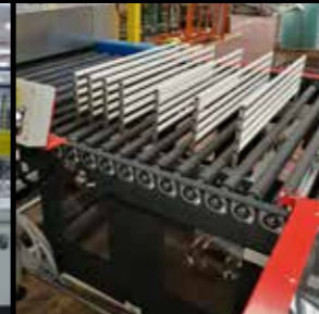
WASHER EMPTYING UNIT
